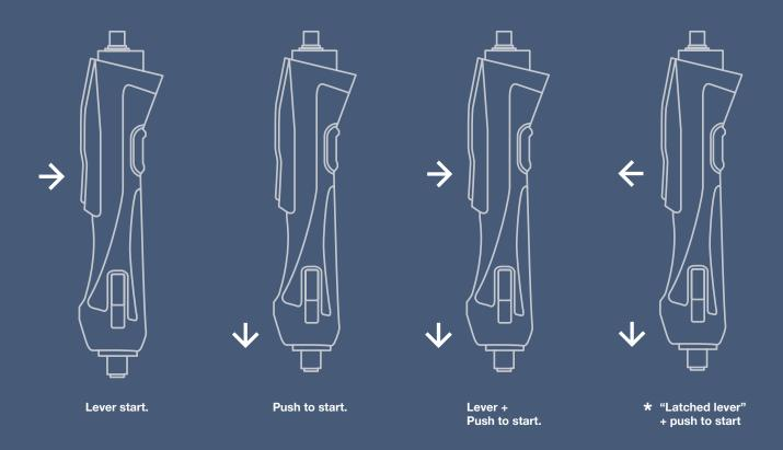
\* The "latched lever" + push to start mode allows the screwdriver to work without need to keep the lever pressed. For safety, the screwdriver activates only when pushing on the bit. In this mode, the first pressure applied to the lever starts the screwdriver until clutch shuts off, whereas a second pressure can eventually stop it before the working cycle is completed.
